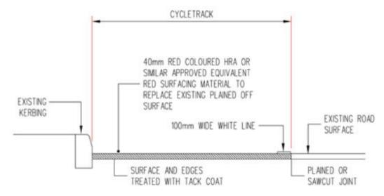
Figure 2-39: Typical cycle track surfacing detail form the National Cycle Manual
