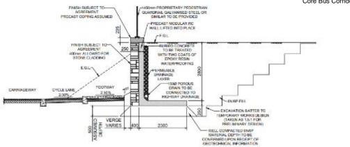
Figure 3-14: Proposed retaining wall plans
