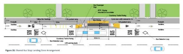
Figure 2-38: Extract of the BCPPDGB, displaying footpath, cycle track, and bus lane arrangements.
