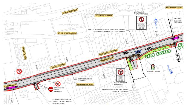
Figure 2-1: Extract 1 from General Arrangement Drawing
