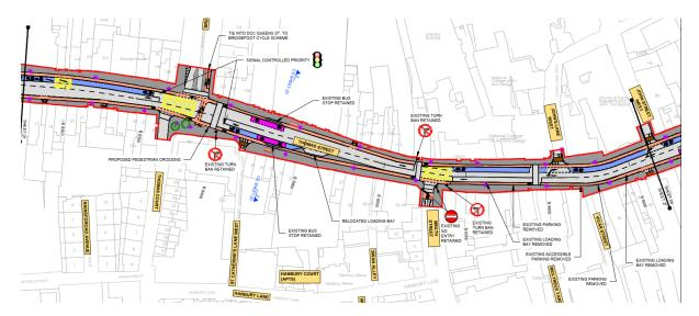
Figure 2-15: Extract 3 from General Arrangement Drawing
