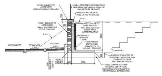
Figure 3-16: Proposed retaining wall detail
